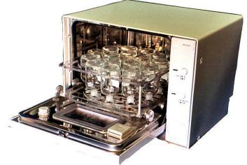
use. Install bottle washer on the bench or on rollaway cart, attach quick disconnect fill/drain hose to faucet and turn on hot water. Push DI hose onto DI valve, fill the reservoir with DI water then turn the DI valve on. To start washing just add soap and BOD bottles. In approximately 25 minutes you will have sparkling clean DI rinsed BOD bottles. 115V/60Hz.
